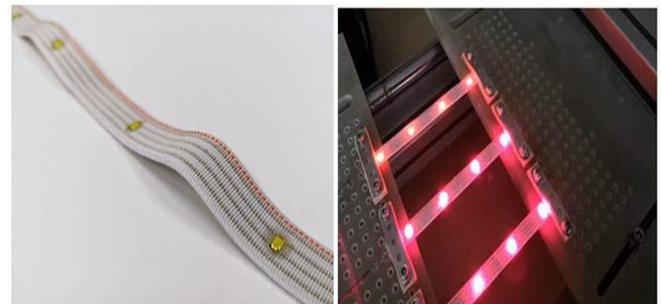
Fig. 5 Conductive stretchable textile ribbons with integrated LED and these ribbons after 4500 stretching cycles[16]
