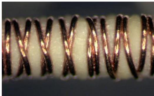
Fig 1. Elastic electroconductive yarn
