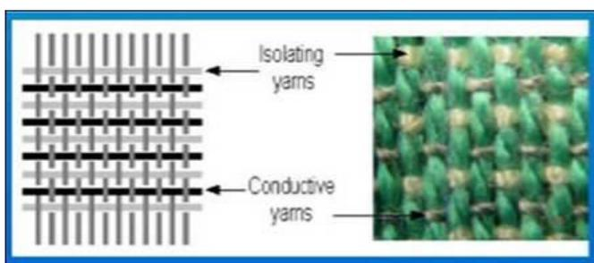
Fig.2 Conductive yarns in the fabric structures
